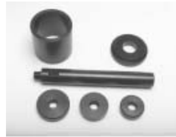
Linkert Venturi Removal Tool This Colony designed tool is precision machined from steel and heat treated for durability. This tool will easily remove the most stubborn venturis and includes set of 3 interchangeable adaptors to service all Linkert carbs. NOTE: The use of an arbor or hydraulic press is strongly recommended. Stock No. 2701-6
